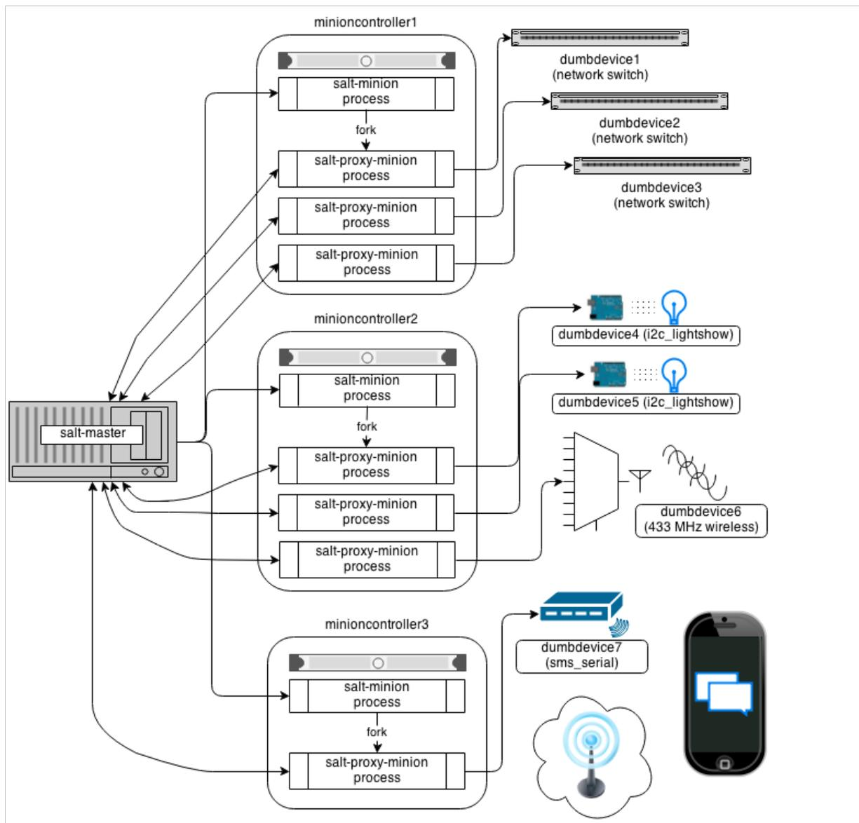
The key thing to remember is the left-most section of the diagram. Salt's nature is to have a minion connect to a master, then the master may control the minion. However, for proxy minions, the target device cannot run a minion, and thus must rely on a separate minion to fire up the proxy-minion and make the initial and persistent connection.
